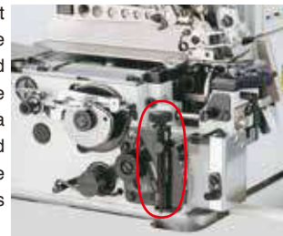
Differential-feed micro-adjustment mechanism
